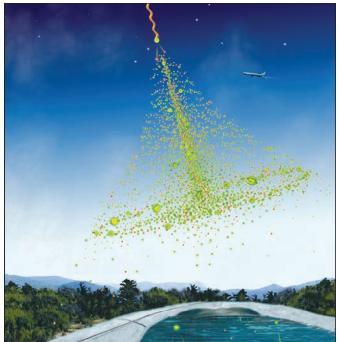
Fig. 1a. The principle behind the Milagro gamma-ray observatory. A high-energy cosmic gamma ray generates a shower of secondary cosmic rays, which are detected via Cherenkov radiation in the water. (Courtesy Aurore Simonnet, Sonoma State University.)
