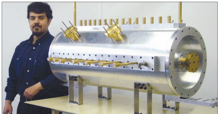
Nader Alharbi and the "cold" (low-level RF power) model built in Saudi Arabia. (Courtesy F Gerigk.)
