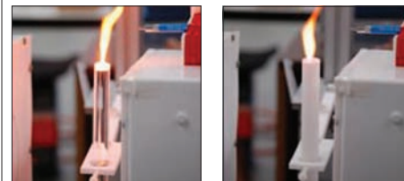
A solution of 3% sodium chloride burns in a Pyrex test tube (left) and a PTFE tube (right) when ignited in the presence of 13.56 MHz RF radiation (Roy, Rao and Kanzius 2008).
